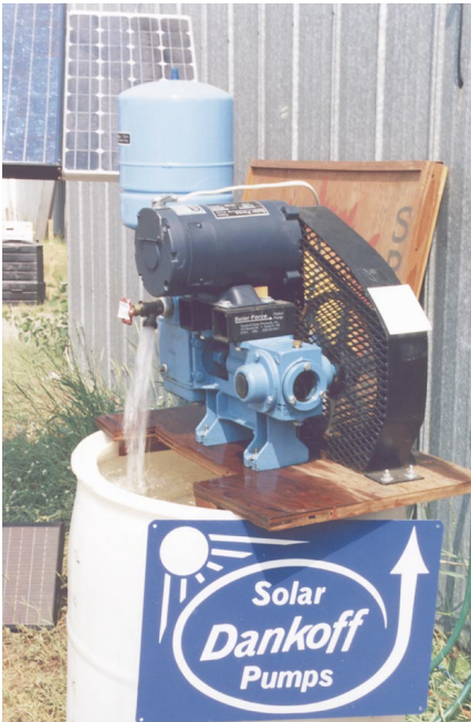
Above: New products, like this PV-powered piston pump, were on working display.
